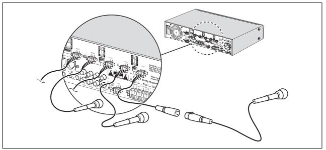
figure 4.3: Connecting microphone inputs
